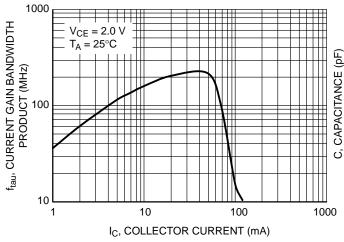
Figure 2. Current Gain Bandwidth Product vs.
