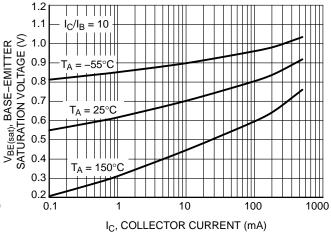
Figure 7. Base Emitter Saturation Voltage vs.
