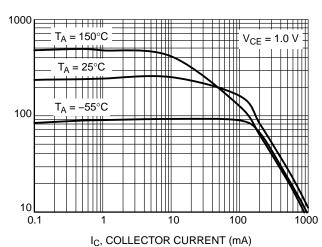
Figure 5. DC Current Gain vs. Collector Current
