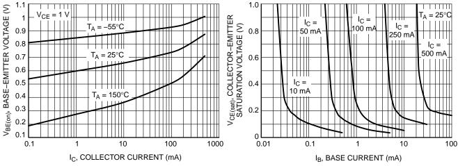
Figure 8. Base Emitter Turn-ON Voltage vs.
